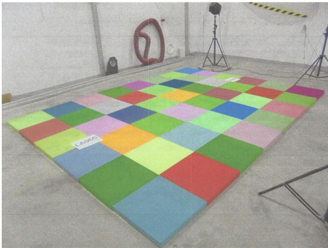
Pic. 1. Photograph of sample LA679, Fluffo Soft soft, acoustic wall panels, in the reverberation chamber at the Laboratory of Vibro-acoustic Testing, Environmental CTO S.A.
